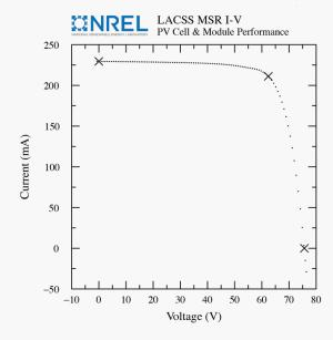
$$\begin{split} &V_{oc} = 75.66 \ V \pm 0.86\% \\ &I_{sc} = 0.2296 \ A \pm 0.66\% \\ &Fill \ Factor = 75.86\% \pm 1.74\% \\ &Efficiency = 19.80\% \pm 1.61\% \end{split}$$
